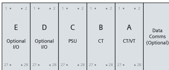
Rear View: Arrangement of terminals and modules
